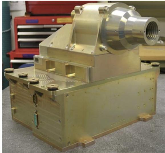
Figura 3.4: Instrumento ECT-REPT. (D. N. Baker, Kanekal, Hoxie, Batiste et al., 2013).
